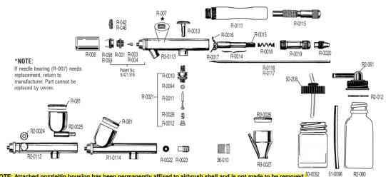
NOTE: Attached nozzle/tip housing has been permanently affixed to airbrush shell and is not made to be removed. \$0.000
